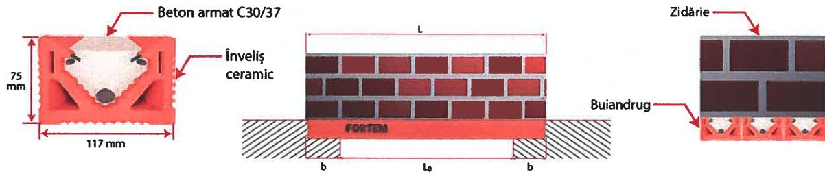
(beton armat - reinforced concrete; invelis ceramic - ceramic coating; zidarie – masonry; buiandrug – lintel)
